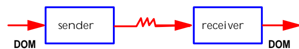
Figure 9. The sender and receiver Xbean abstract the communication of XML over the wire.
