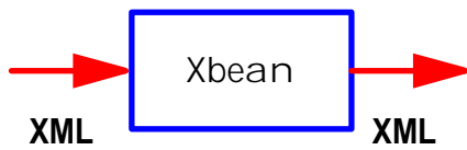
Figure 1. An Xbean consumes XML as input, processes it and then produces XML as output.
